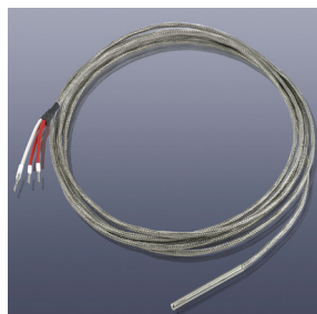
Temperature sensor Pt100 type MIL-TP2 / ø 4 x 50mm
